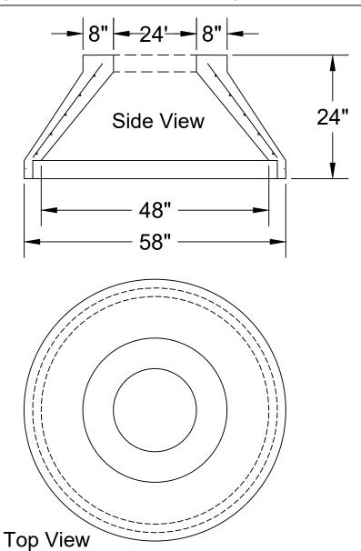
28 Day, 5,000 PSI Concrete G-60 #4 Rebar @ 12" o.c.e.w. Meets ASTM C-1227, 990, 923 H-20 Traffic Rated +/- 1/2" Tolerance Print not to scale
