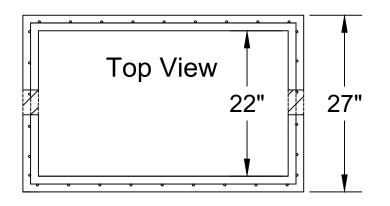
28 Day, 5,000 PSI Concrete #3 Rebar on 12" Centers Print Not To Scale
